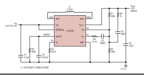
Low Profile Li-Ion to 3.3V at 300mA Converter with Automatic Burst Mode Operation
