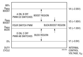
Figure 2. Switch Control vs Internal Control Voltage,  $V_{\mbox{CI}}$
