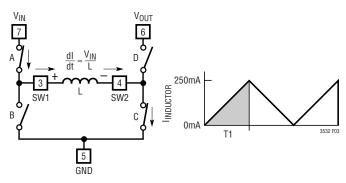
Figure 3. Inductor Charge Cycle During Burst Mode Operation
