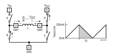
Figure 4. Inductor Disharge Cycle During Burst Mode Operation
