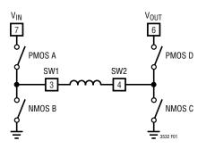
Figure 1. Simplified Diagram of Output Switches
