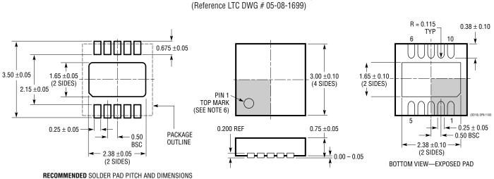
**DD** Package 10-Lead Plastic DFN (3mm × 3mm)
